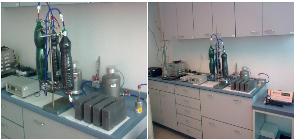
Figure 2. Pictures of experimental setup type I used for measurement of charcoal ability to capture radon. The charcoal was given into three PET bottles. The radon activities in the input and output were monitored by two ionization chambers. The activity of radon in the air of laboratory was continuously detected by monitor Alphaguard (providing also temperature, relative humidity). As the emanation source Pylon A-2000 was used ( ^{226}\text{Ra}/^{222}\text{Rn} emanation source).
