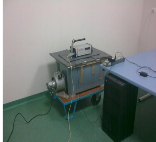
Figure 8. View of empty charcoal container with both holes used as input and output for air flowing into the charcoal (left picture). The whole apparatus (air pump, charcoal container, radon monitor Alphaguard) is presented in right picture.
