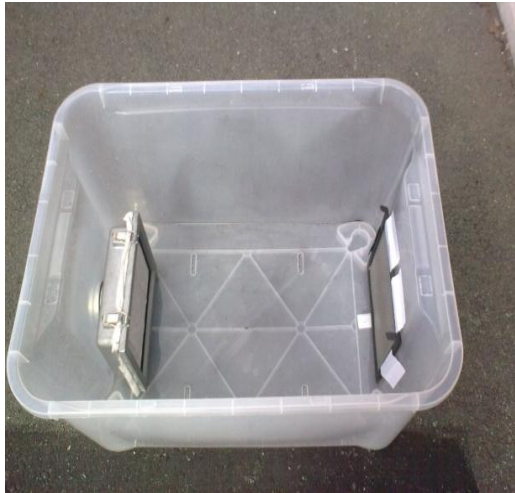
Figure 8. View of empty charcoal container with both holes used as input and output for air flowing into the charcoal (left picture). The whole apparatus (air pump, charcoal container, radon monitor Alphaguard) is presented in right picture.
