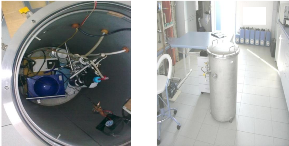
Figure 6. Pictures of experimental setup type II used for measurement of radon suppression by charcoal trap for small volume without any air ventilation. As charcoal container the PET bottle was used. The measurements were performed with charcoal placed inside and outside of the steel vessel, respectively.
